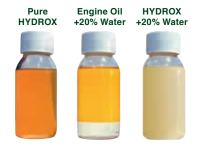
Using HYDROX BIO lubricants dramatically reduces wear to sterntube bearings in the event of seawater ingress.
