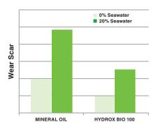
HYDROX BIO lubricants are biodegradable lubricants based on synthetic esters, developed primarily for use in sterntubes and bearings where water ingress may occur. The products provide:
